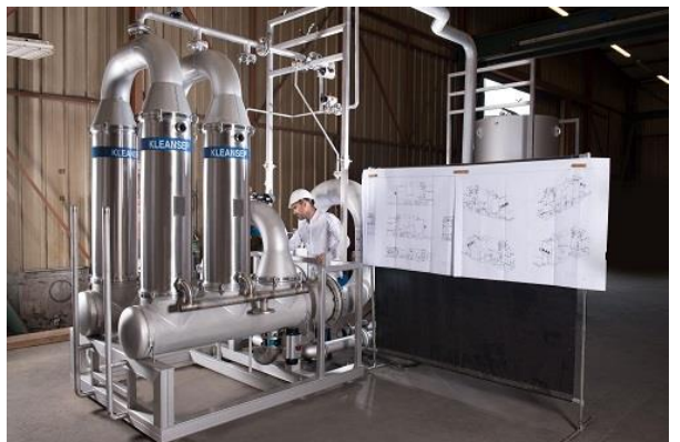
Industrial equipment and process engineering: filtration skid
