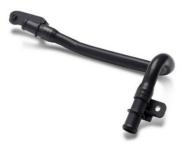
Solvay's new Ryton® PPS extrusion series is designed to complement proven Ryton® PPS injection molding materials for use together in demanding automotive cooling line assembly applications. The stiffness of these grades varies between 1500 Mpa (218 ksi) and 2500 Mpa (363 ksi) to fulfil requirements of flexible tubes with different wall thicknesses and diameters or for post-extrusion thermoforming. Photography and graphic courtesy of Solvay.
