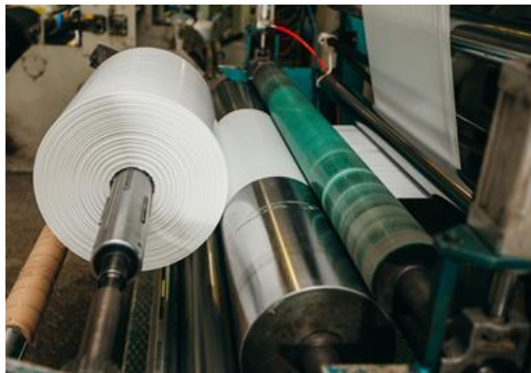
PHOTO: DOW CORNING™ MB25-235 Masterbatch Reduces the Coefficient of Friction (COF) of Low Density Polyethylene (LDPE) Film to Optimize Flexible Packaging Production
