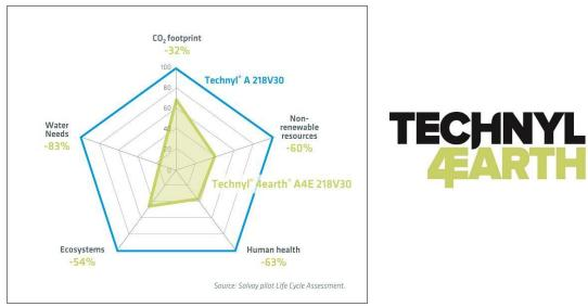
The cradle-to-gate environment footprint of Technyl<sup>®</sup> 4earth<sup>®</sup> is significantly reduced vs. prime Technyl<sup>®</sup> PA6.6. Diagram: Solvay Performance Polyamides
