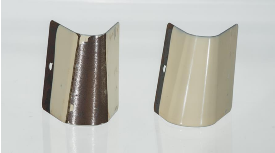
PHOTO: Mandrel Bend Test Comparison After Five Days at 120 C Showing that the Control Sample (left) Cracked and Delaminated, While the SiVance C2010 Resin Sample (right) Passed
