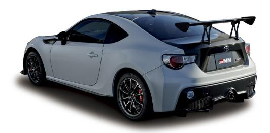
Toyota's special edition 86 GRMN sports car is the first production vehicle to feature a rear quarter window in polycarbonate (PC) material (LEXAN™ resin) with a proprietary coating solution from SABIC − EXATEC™ plasma technology. The high impact strength and optical clarity of LEXAN resin combines with the advanced abrasion resistance of the EXATEC coating to meet regulatory requirements for driver visibility.
