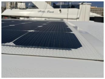
Highly transparent photovoltaic (PV) frontsheets extruded by Amcor, using Solvay's Halar® 500 ECTFE resin, enabled Solbian Energie Alternative to innovate solar panels that integrate directly into a boat's deck. Solvay's lightweight, durable ECTFE resin enabled Amcor's frontsheets to offer a highly-transparent, textured non-slip surface that could withstand both harsh marine conditions and frequent foot traffic. Photo courtesy of Solbian Energie Alternative.
